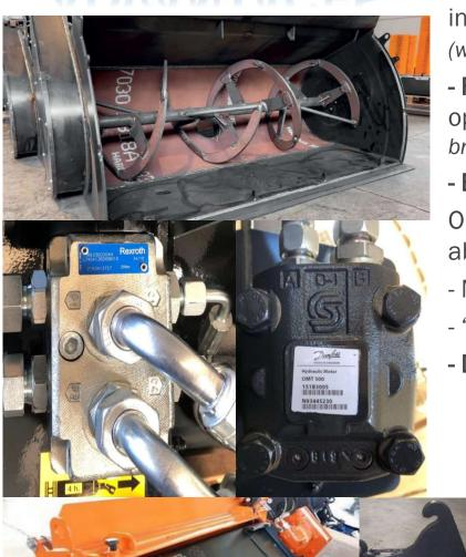
Mixing auger made of **HARDOX 500Tuf**.
